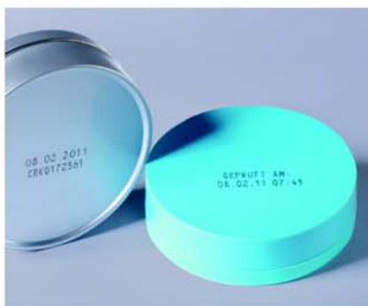
Printing with quick drying ink on metal and plastic (Version MP).
